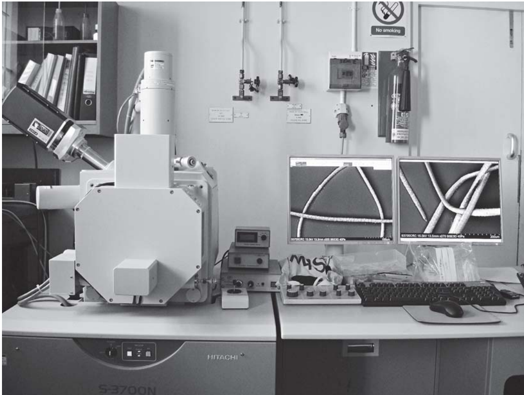
Figure 1. The variable pressure scanning electron microscope (VP-SEM) at the British Museum which was used for the identification of plant materials from the selected ancient Egyptian sandals.
